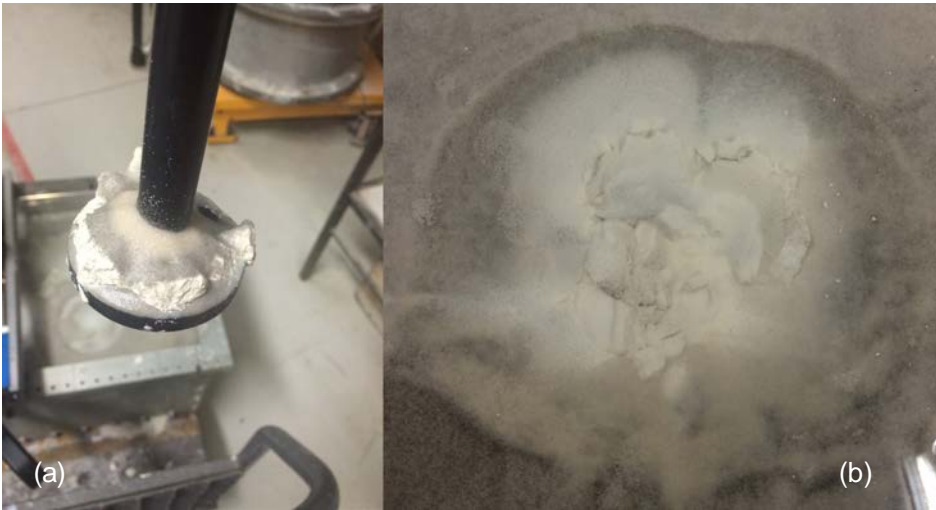
FIGURE 5. Evidence of soil flow through holes of spudcan H: (a) Soil column left on extracted spudcan; (b) Soil column on site
