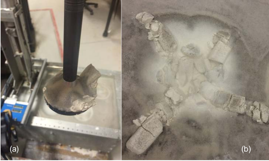
FIGURE 4. Evidence of soil flow through slots of spudcan S: (a) Soil column left on extracted spudcan; (b) Soil column on site
