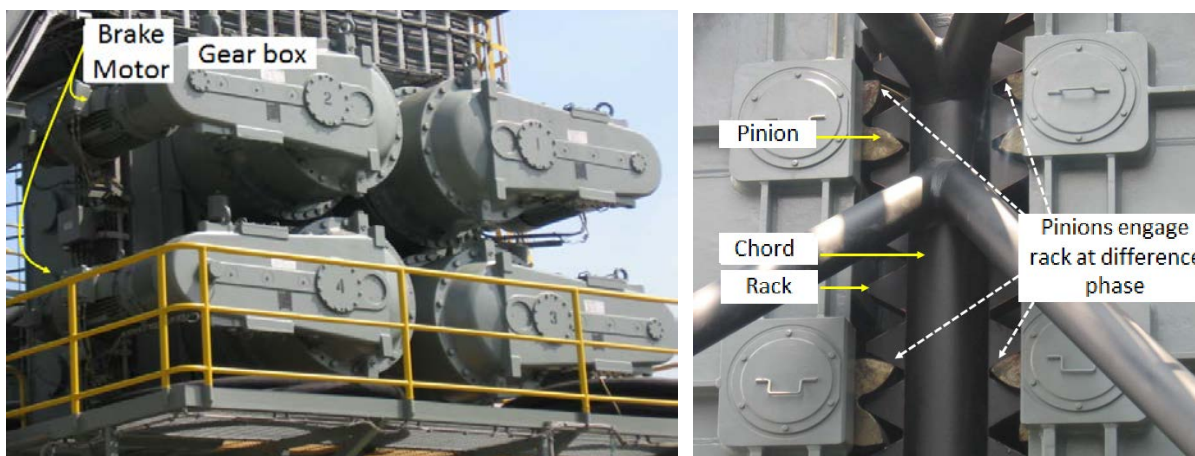
Fig 1: (left) Jacking system with four jacking units per chord (right) Rack and Pinion System
