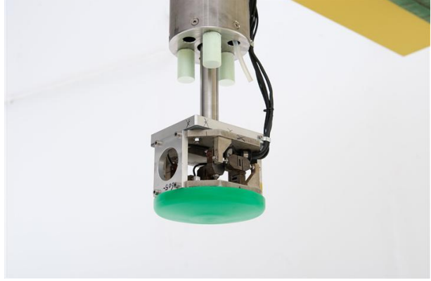
Photo 2: leg tip with 6 DOF force measurement frame and HMPE 1000 spudcan (green)
