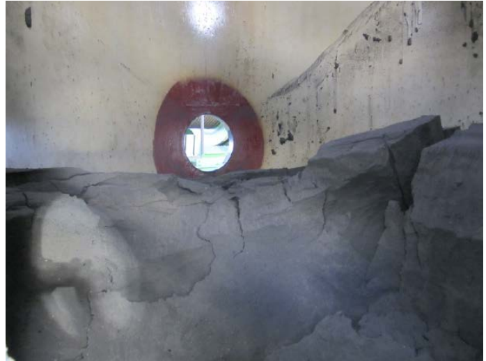
Figure 10: remoulded London Clay at the interior of the legs of NEPTUNE
