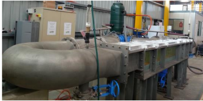
Figure 2. The small O-Tube facility used for the testing.
