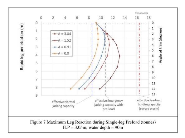
The results for the single leg preload assumption are presented in Figure 7. The rig move team can now focus their attention on one leg at a time, and there are some key advantages:
