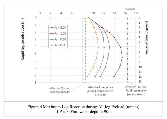
The simplified RPL method assumes a bow leg penetration with the rig rotating about the stern legs and that the stern leg spudcans have no moment capacity. For these simplified calculations, an initial leg penetration (ILP) of 3m was assumed. The airgap (A) was varied from 0m to 3m. The results for the all-leg preload assumption are presented in Figure 6.
