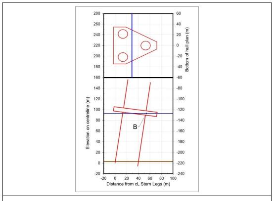
Figure 5 Location of centre of buoyancy due to a bow leg RLP with an 8° loss of trim The location of the hull centre of gravity is dependent on amount & location of preload
