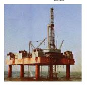
The Transocean 1, built in Germany in 1965 is reportedly the first jack-up designed specifically to operate in the North Sea. It had six tubular legs, each fitted with one rack forward and one rack aft. After its North Sea life it was converted to a production facility in the Arabian Gulf called the Deutag 1.
