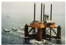
There are two rigs included in this category, the Transworld 61 (1970) and the Transworld Rig 60 (1971). The Transworld Rig 60 is a jack-up submersible. Makes sense; why not extend the water depth range of the submersible type rig by sticking a modified jack-up on top of it?
