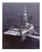
The Offshore Rig 52, built in 1955 had fourteen legs and was retired in 1980. The unit was comprised of two jack-ups that were welded together.
