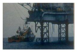
On 23<sup>rd</sup> June 1988 the ship "Irving Forest" was travelling through the North Sea, with good visibility, but with an unmanned wheelhouse, when it collided with the Glomar Labrador 1, knocking out half of one leg. Fortunately, the rig survived and there were no injuries. The wheelhouse was unmanned because the relief officer was always late, so the officer being relieved decided to show him what for, and leave the wheelhouse unattended.
