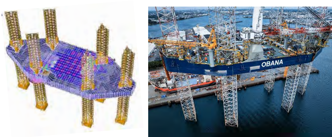
Figure 7: Hull stress during pre-loading (left), jacking trials (right)
