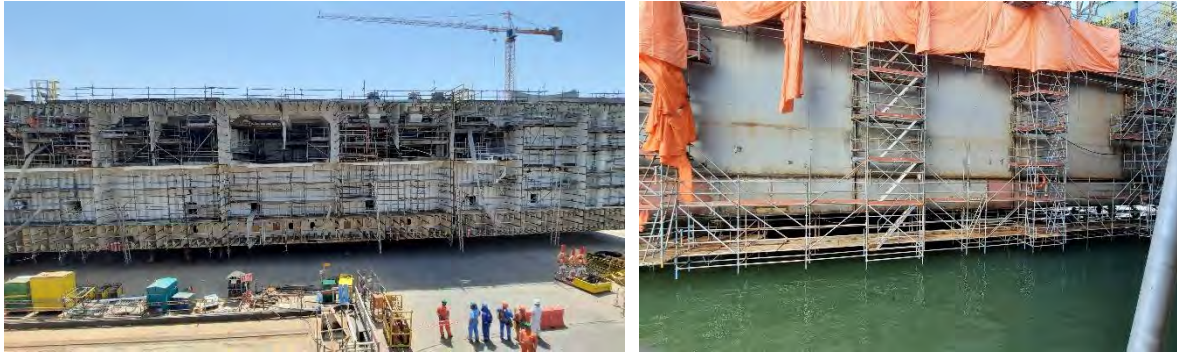
Figure 8: Midsection fabrication (left), preparation of GII and GIII transom (right)
