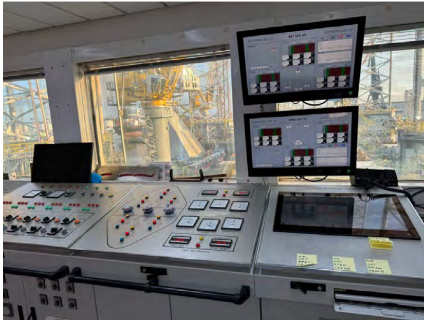
Figure 17b Jacking control system of OBANA after the retrofit
