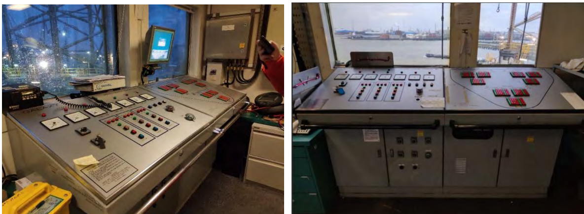
Figure 17a Jacking control system of Galaxy II and Galaxy III before the retrofit
