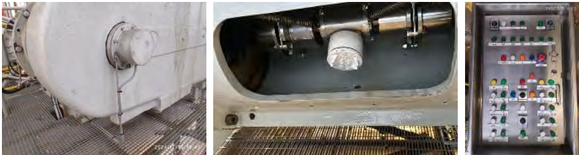
Figure 16 New control features such as RPD & leg load monitoring and emergency jacking controls
